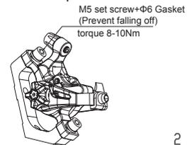
2. Assemble the caliper and adapter onto the rear fork.
