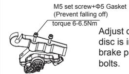
Adjust disc to make sure the disc is in the middle of 2 brake pads, then tighten the bolts.
